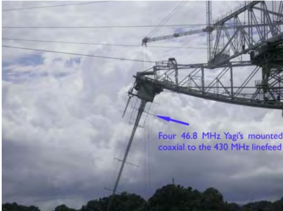
Figure 3: The 430 MHz UHF and 46.8 MHz VHF radars.
