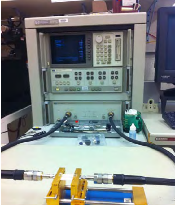
Figure 3: The microstrip is fastened into an adapter that allows the network analyzer to transmit electric signals across it.
